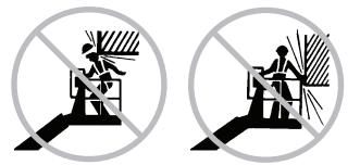
Be aware of crushing hazard when grasping the platform guard rail.
